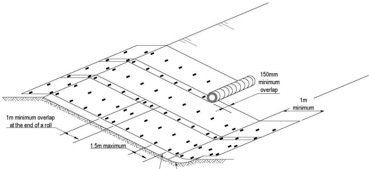
Anchor type is to be to the manufacturer's recommendation. Anchor spacing is to be to the smaller of the manufacturer's recommendation or the dimensions shown.
