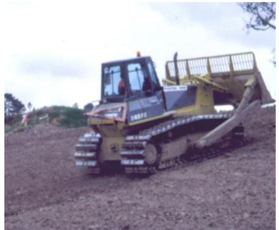
Figure 38: Surface roughening with bulldozer
