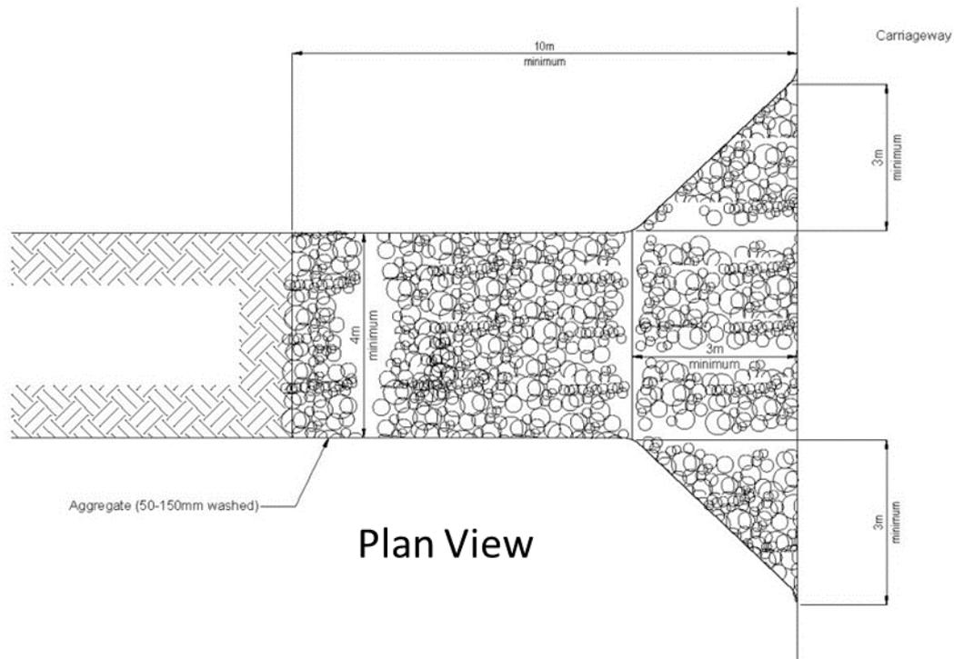
**Figure 35: Stabilised entranceway**
