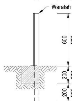
**Figure 83: Step-by-step installation of a silt fence**
