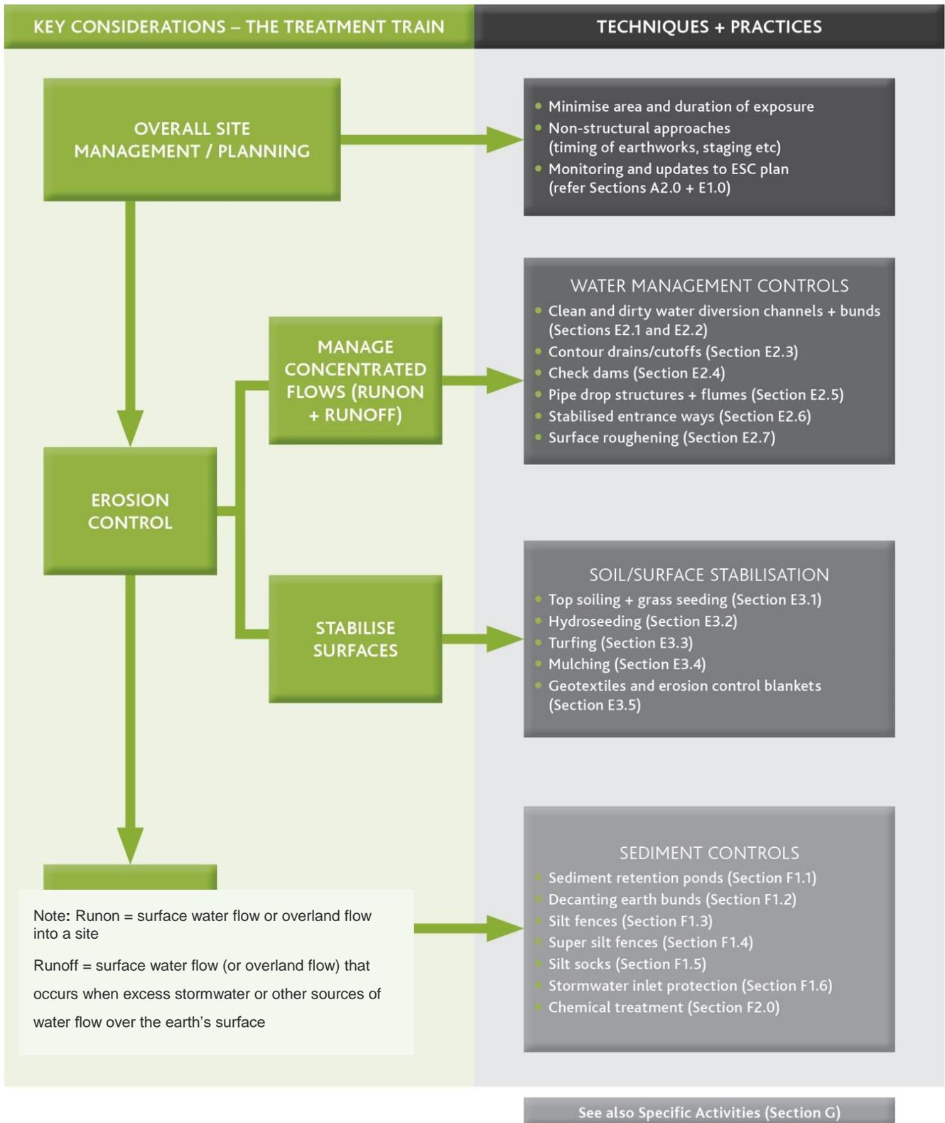
Figure 9: Process to select the best practice option(s) and develop an ESC Plan for development / construction
