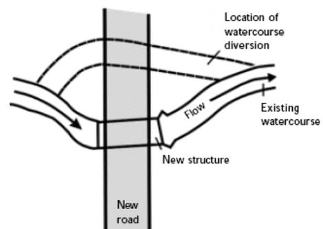
**Figure 121: Re-establishment of flow in original channel**
