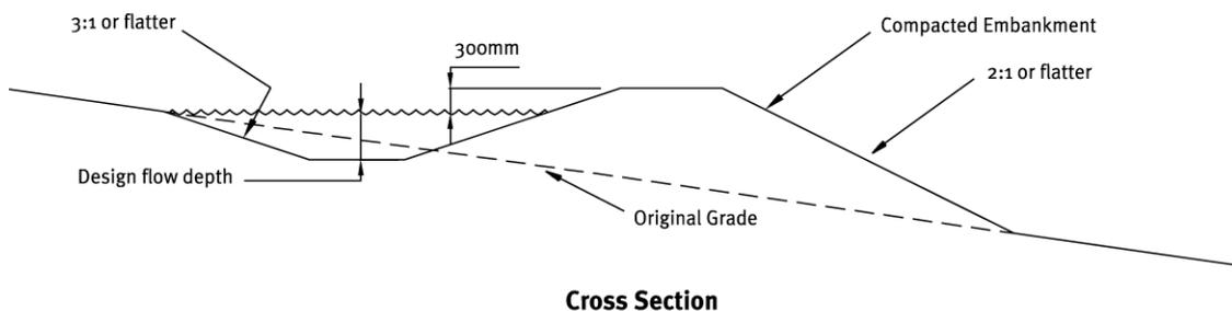
**Figure 18: Cross-section of a dirty water diversion**
