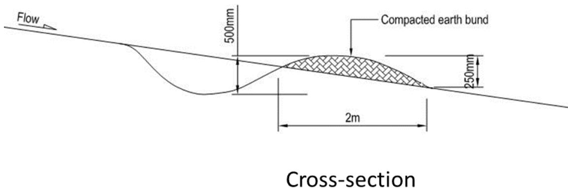
**Figure 23: Contour drain cross-section**
