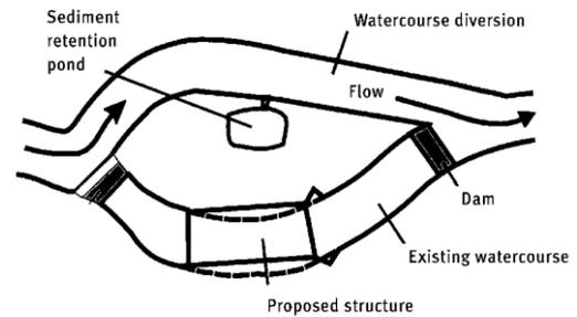
**Figure 119: Dewatering construction area into a sediment pond**
