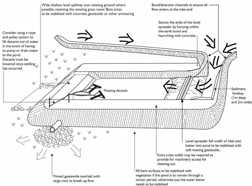
**Figure 64: Schematic of a sediment retention pond**
