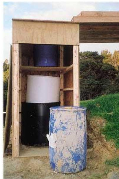
**Figure 99: rainfall activated flocculant treatment device**
