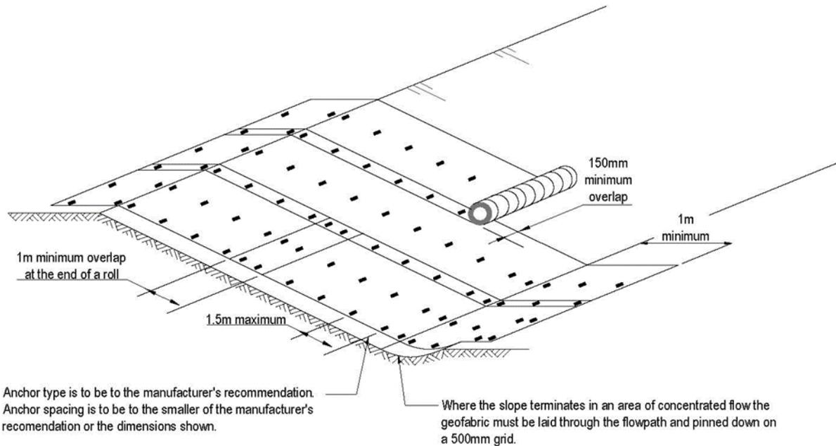
**Figure 58: Geotextile design – outfalls**
