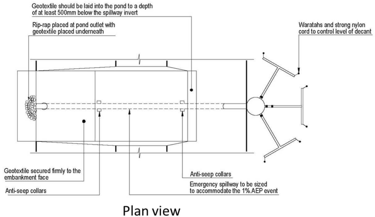
Figure 73: Sediment retention pond for 3 to 5 ha catchment
