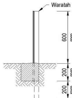
**Figure 83: Step-by-step installation of a silt fence**
