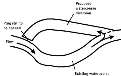
**Figure 118: Diversion channel prior to plug removal**
