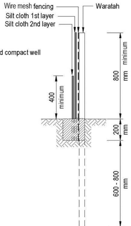
Figure 88: Step-by-step installation of a super silt fence
