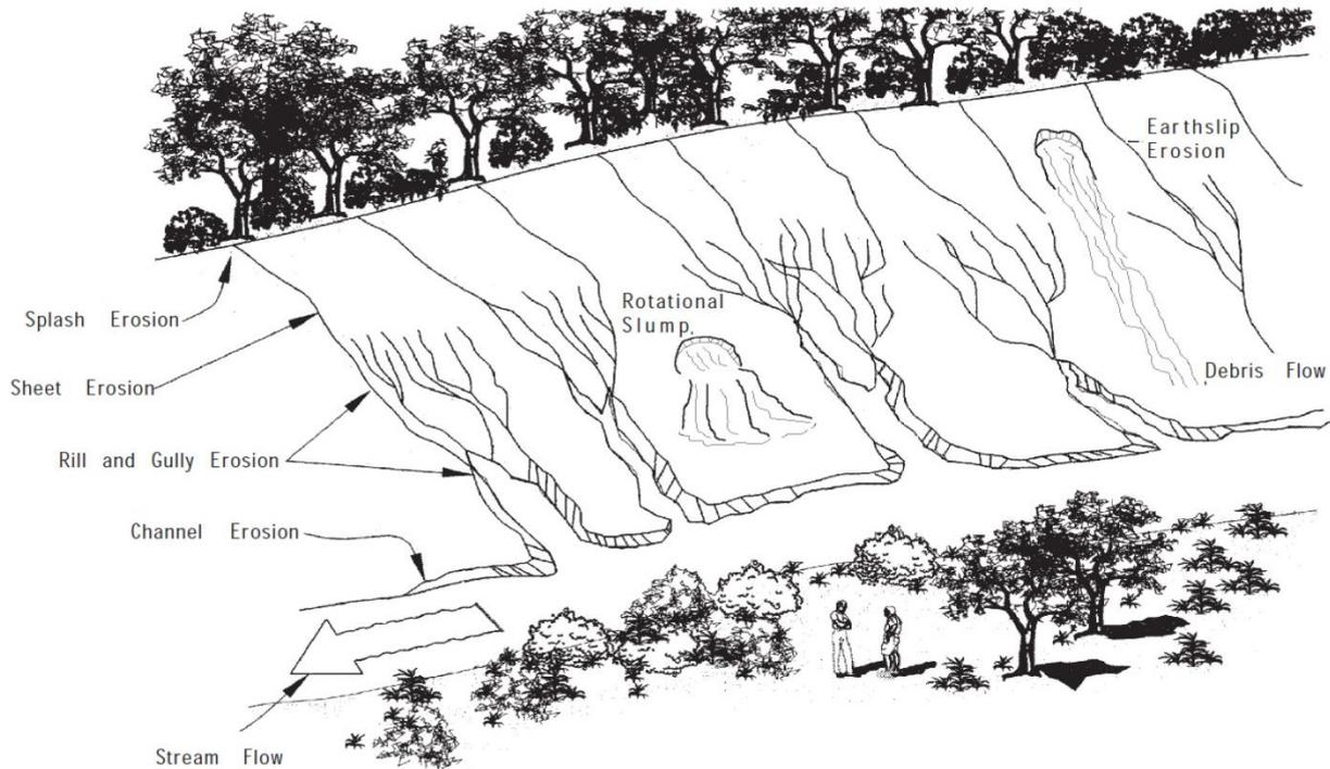
**Figure 5: Types of erosion**
