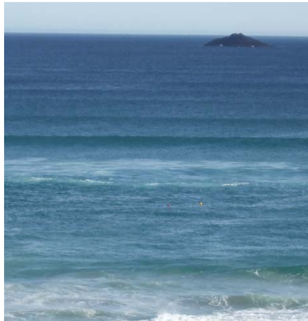
Figure 7.2 One of the signal buoys deployed in the surf zone trough. Note the red buoy is moored and the yellow buoy streams with the current.
