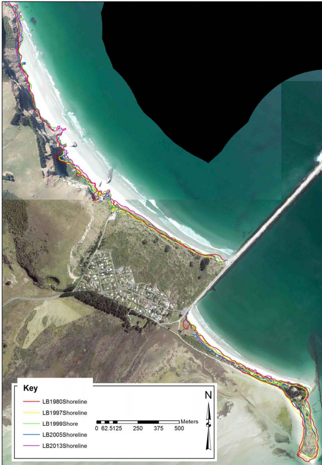
Figure 2.6 Shoreline changes at Aramoana and Shelly Beach plotted from aerial photographs from 1980 to 2013. Base photo is 2013 imagery.
