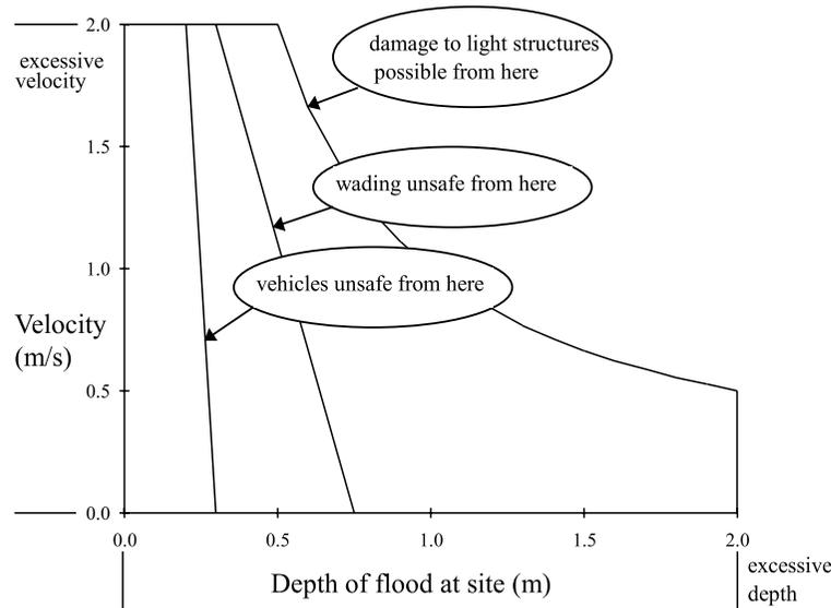
FIGURE 6: HAZARDS RELATED TO FLOOD DEPTH AND VELOCITY
