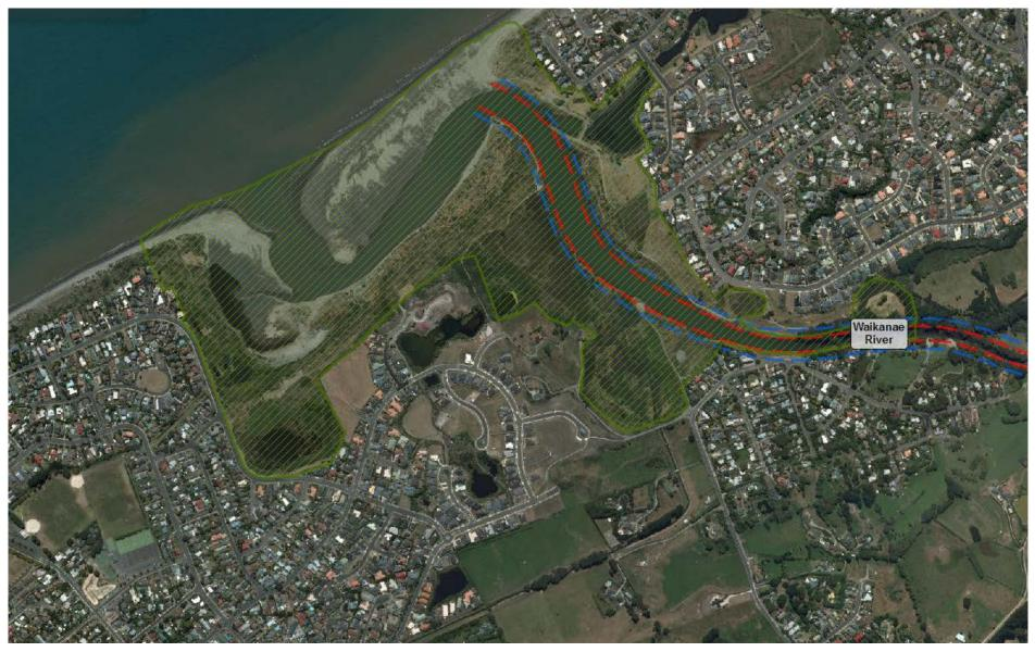
Figure 3-16: View of the application area (dashed blue lines) and design channel alignment (dashed red lines) within the Waikanae Estuary (hatched)
