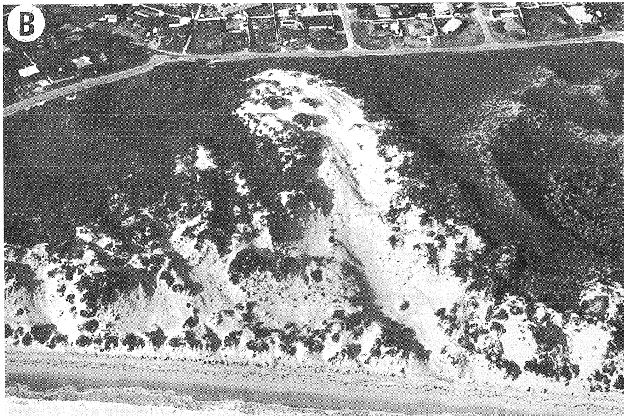
Fig. 10B Elongate trough blowout comprising a deep deflation basin, lateral erosion walls, trailing ridges and a depositional lobe. The blowout has been migrating at 18\text{ m a}^{-1} and the houses are in imminent danger of engulfment (photograph by S. Chape)
