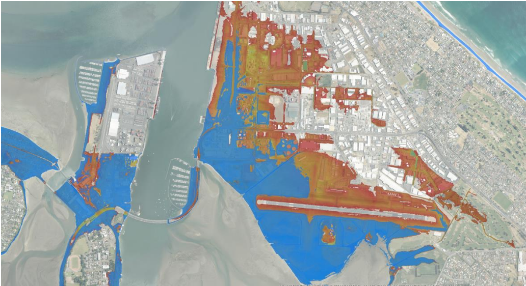
Figure 2-5: Comparison of coastal inundation in Tauranga Harbour estimated from dynamic (left) and bathtub models (right). The scenario modelled was a 1% AEP storm-tide + 1.25 m SLR in Tauranga Harbour Source: Stephens et al. (2018a).
