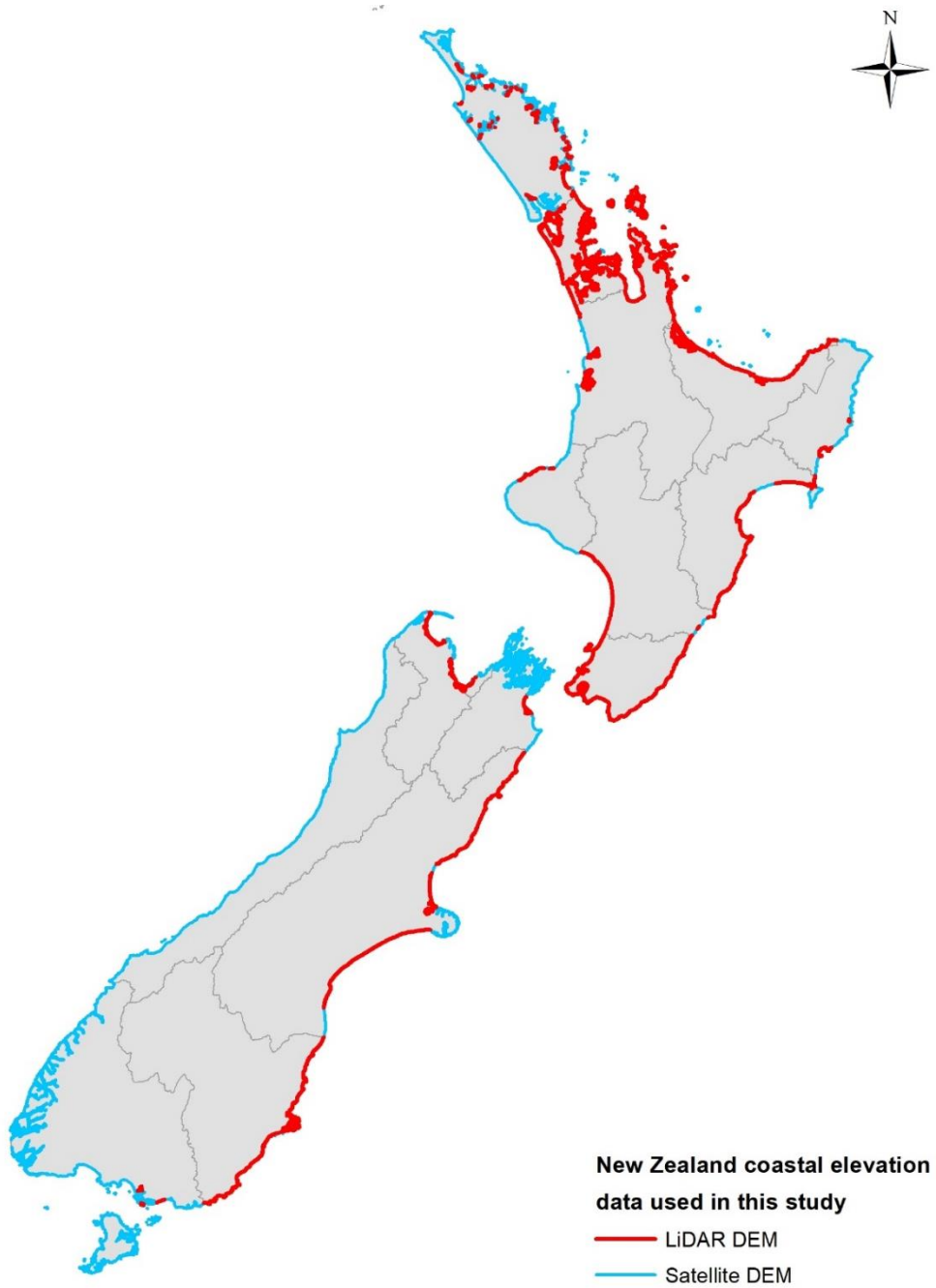
Figure 2-4: LIDAR DEM coverage for New Zealand’s coastline (Note: Satellite DEM provides nationwide coverage).
