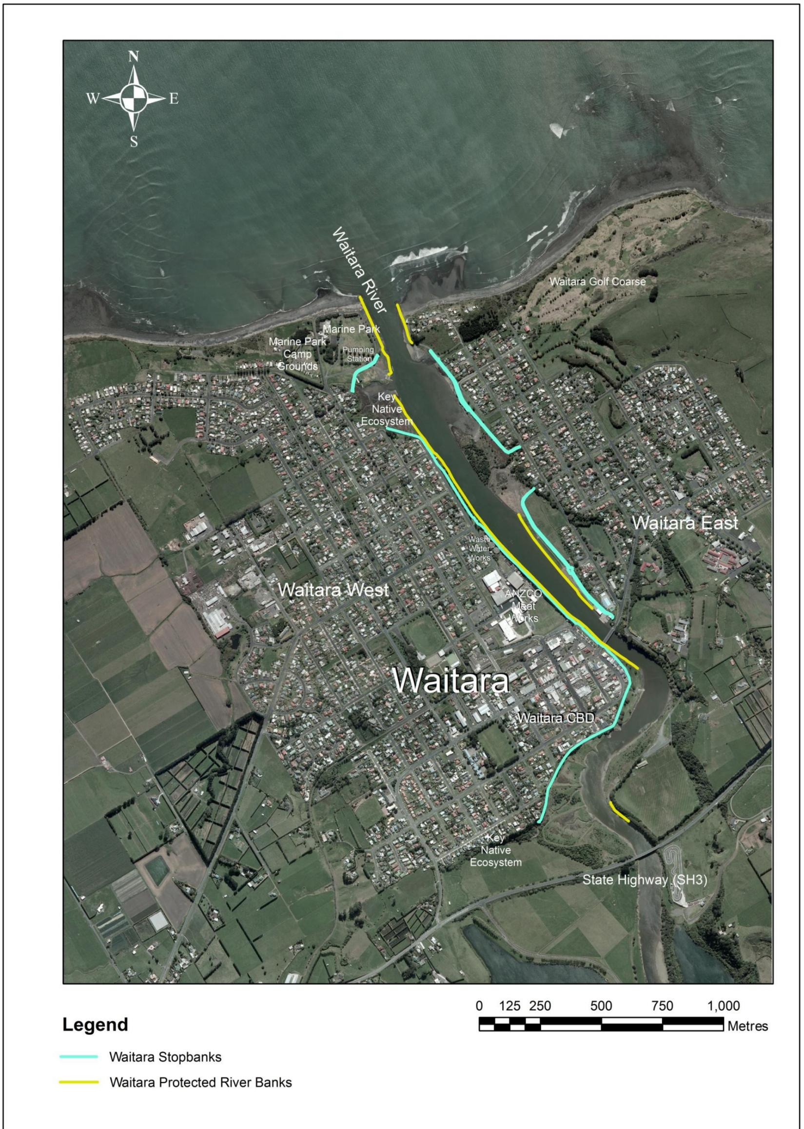
Map 9.9.2 :- Showing Waitara elevations in 1 metre increments in addition to stop banks and armoured river banks.
