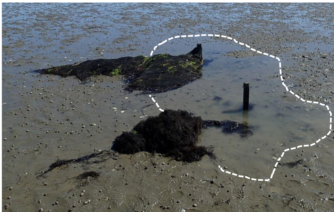
Figure 4: A buried plate where scour has occurred. The plate is buried between the two pegs and a deep scour depression can be seen (white lines). The scour is caused by macroalgae catching and pivoting on pegs with the ebb and flood of the tide. This could have been avoided if the pegs were spaced further apart, a greater distance away from the plate.
