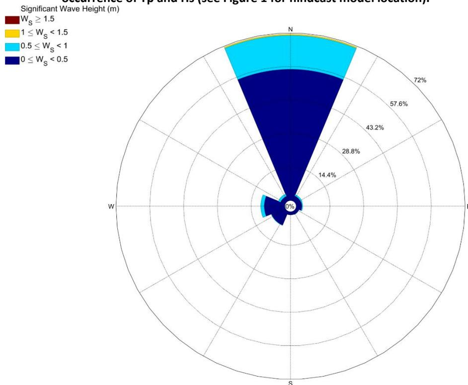
**Figure 15. Wave rose showing distribution of wave events from the MetOcean View hindcast model plotted as the percentage occurrence of Hs and the associated wave direction**
