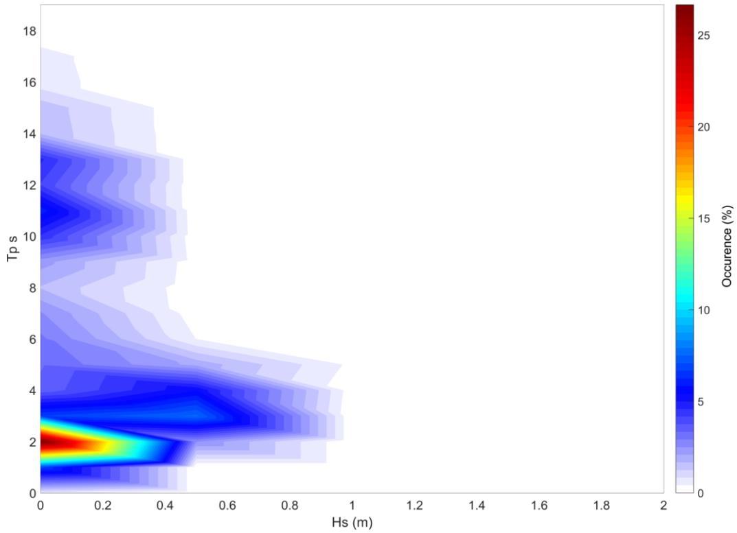
**Figure 14: Distribution of wave events from the MetOcean View hindcast model plotted as the percentage occurrence of Tp and Hs (see Figure 1 for hindcast model location).**
