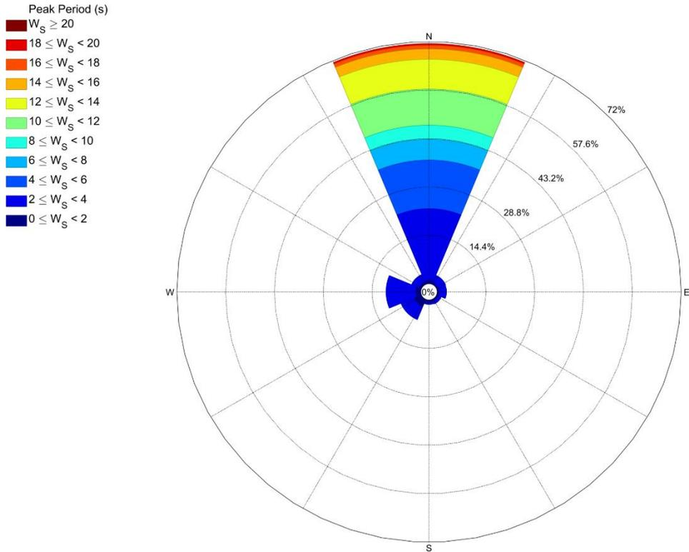
**Figure 16: Wave rose showing distribution of wave events from the MetOcean View hindcast model plotted as the percentage occurrence of  $T_p$  and the associated wave direction.**
