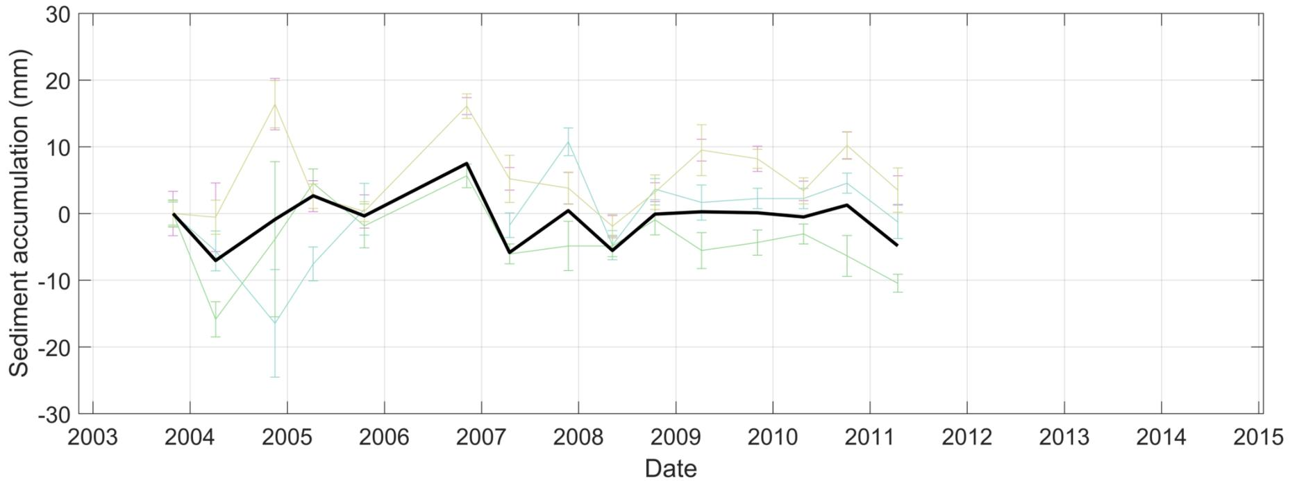
**Figure 12: Sedimentation recorded over the Ponganui Creek Plates.**
