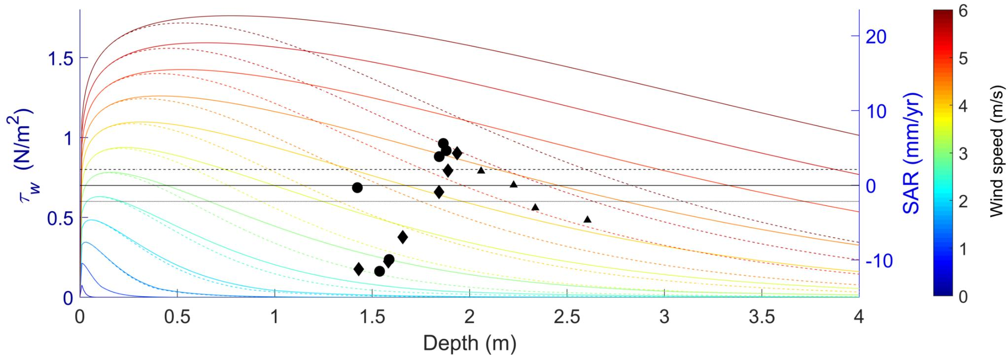
**Figure 18: Modelled  $\tau_w$  for a 100 km fetch (solid coloured lines) and a 25 km fetch (dashed coloured lines) for water depths ranging between 0 and 4 m and wind speeds ranging between 0 and 6 m/s.**
