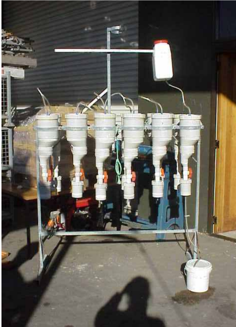
Figure 2. Setting up for a field experiment: chambers used in the field experiments, showing one header tank and collection bucket.
