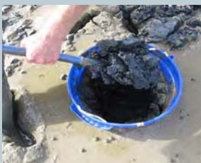
Figure 10 Digging hole to place sediment plate.
