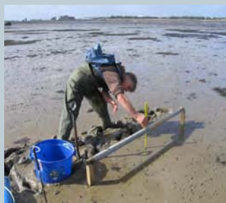
Figure 26 Measuring sediment height - New River Estuary
