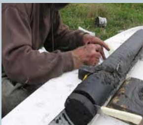
Figure 9 Collecting sediment core and cutting for analysis.
