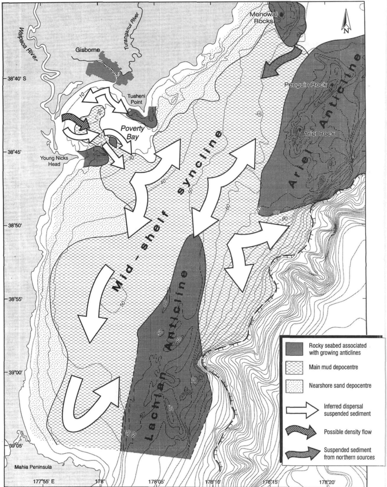
Fig. 10 A model for Poverty Bay mud sedimentation incorporating the structural elements that control the mud depocentre, the main dispersal paths, and the middle shelf mud depocentre.
