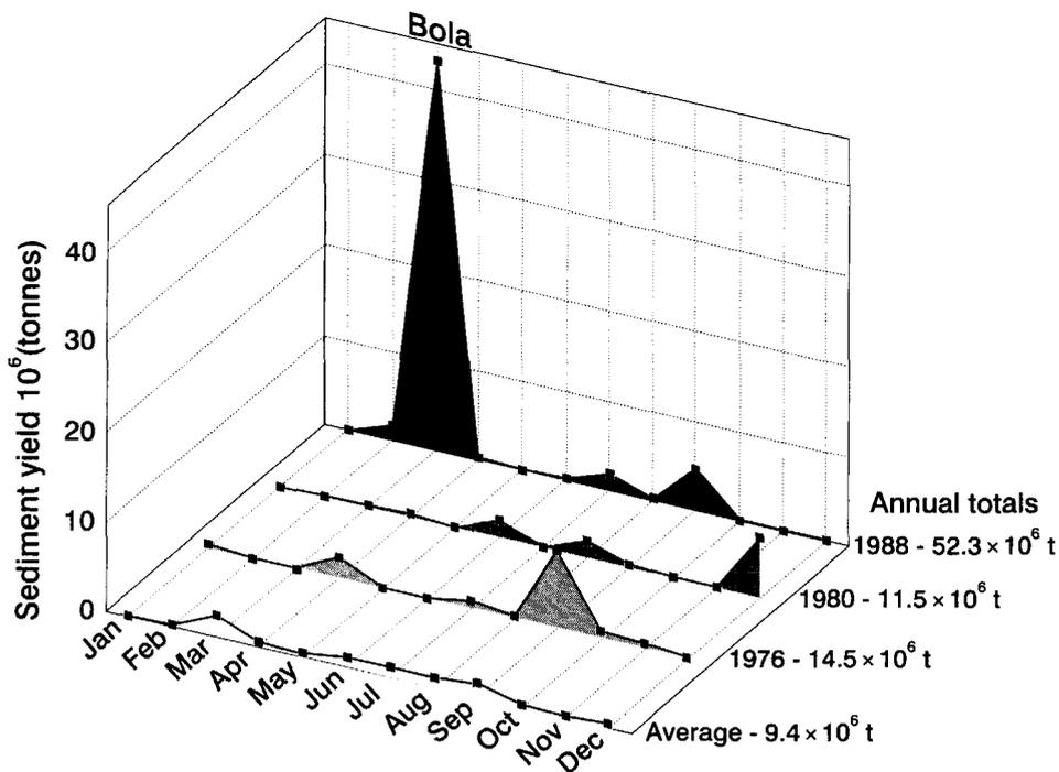
**Fig. 4** Monthly suspended sediment yields (load) for the Waipaoa River for an average year and years of major cyclones, including 1988 when the 100 year storm of Cyclone Bola struck the North Island.
