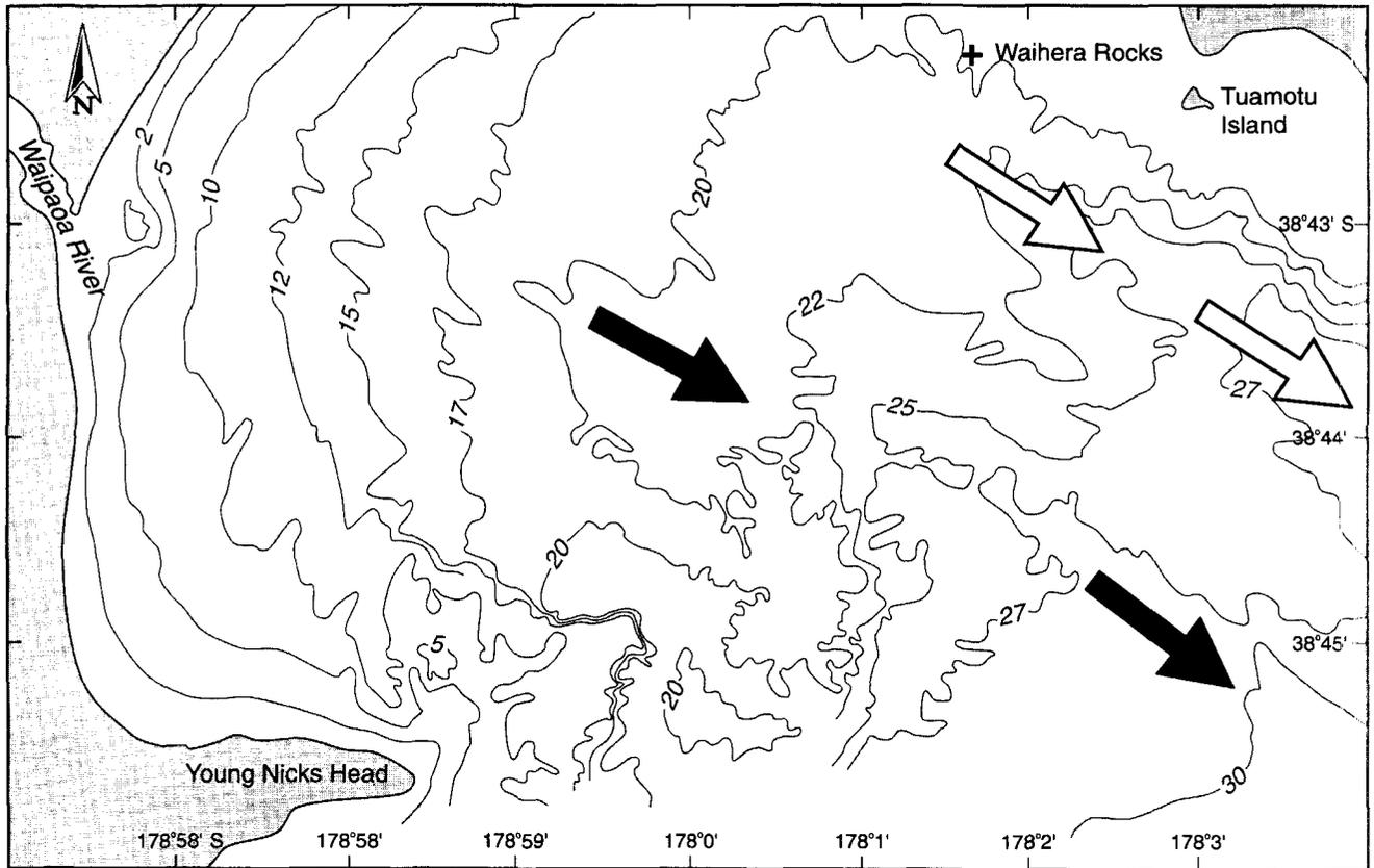
**Fig. 6** Detail of metric bathymetry in southern Poverty Bay outlining the broad trough (solid arrows) leading from the Waipaoa River. The trough in the north of the bay (open arrows) is a relic from when the Waipaoa River discharged in that reach.
