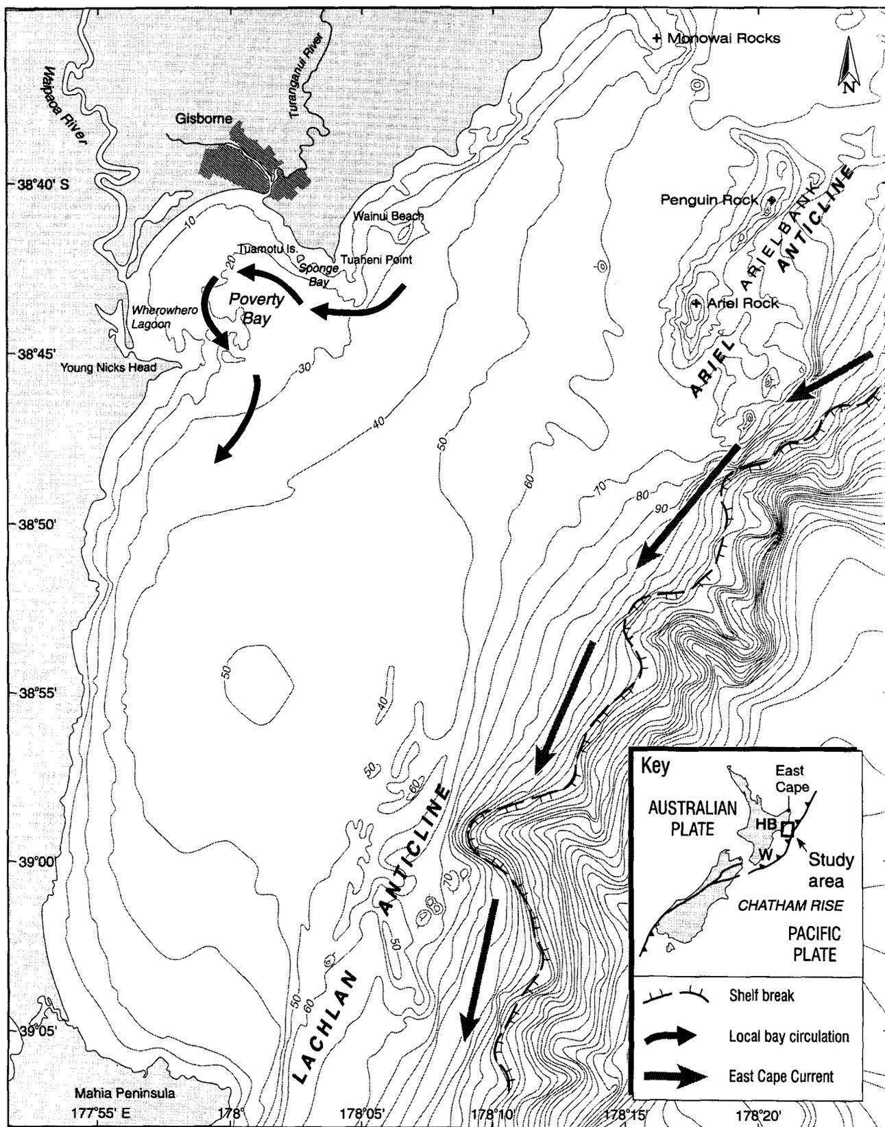
**Fig. 1** Poverty Bay and the eastern continental margin showing metric bathymetry derived from Arron & Lewis (1992) and the main elements of the shelf circulation including the East Cape Current (Heath 1985) and Poverty Bay currents (Miller 1981). *Inset:* The New Zealand plate boundary.
