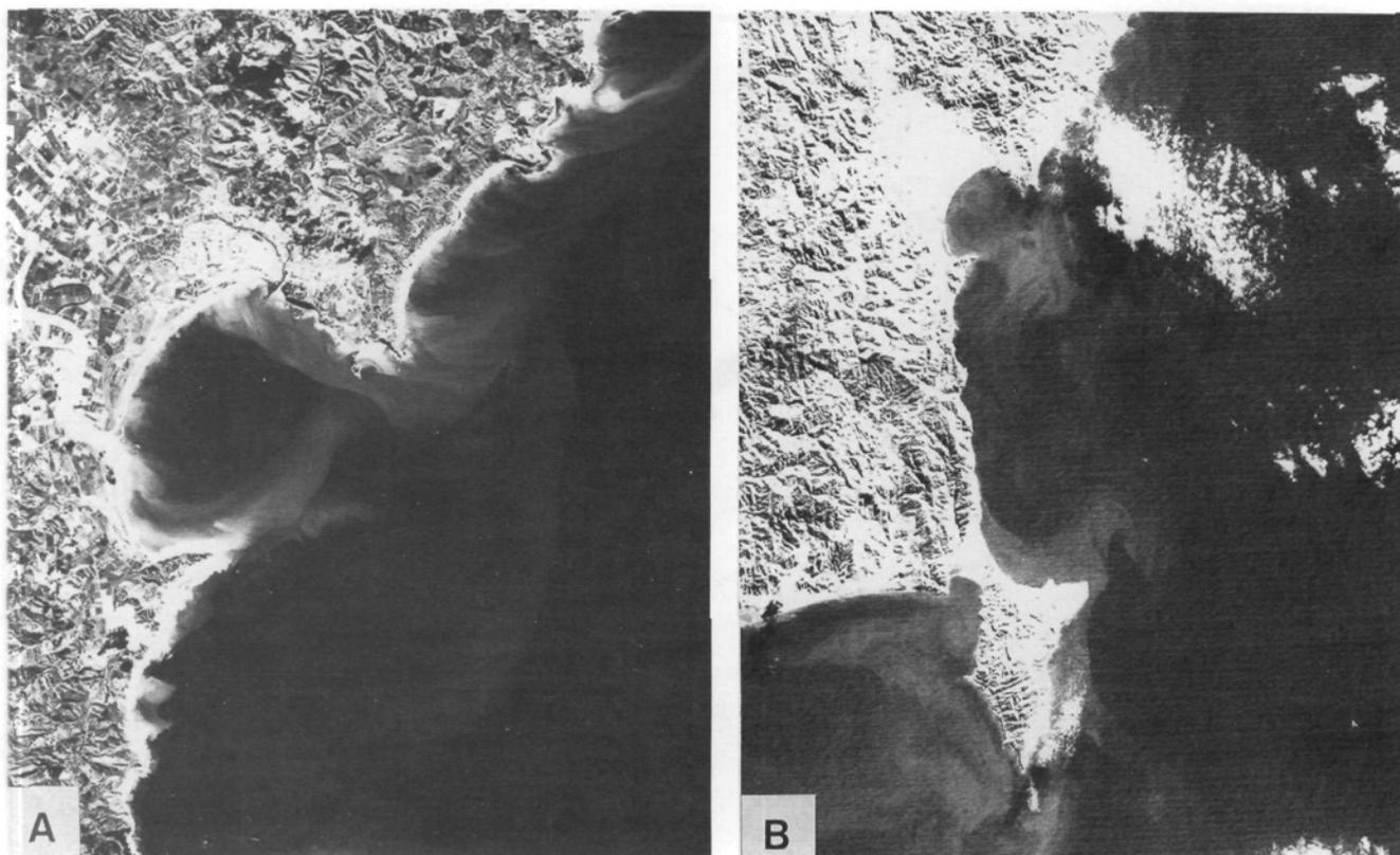
Fig. 5 SPOT (A) and Landsat (B) satellite images highlighting the northward and southward transport of sediment plumes, respectively. (SPOT Image (CNES) supplied by Landcare Research.)
