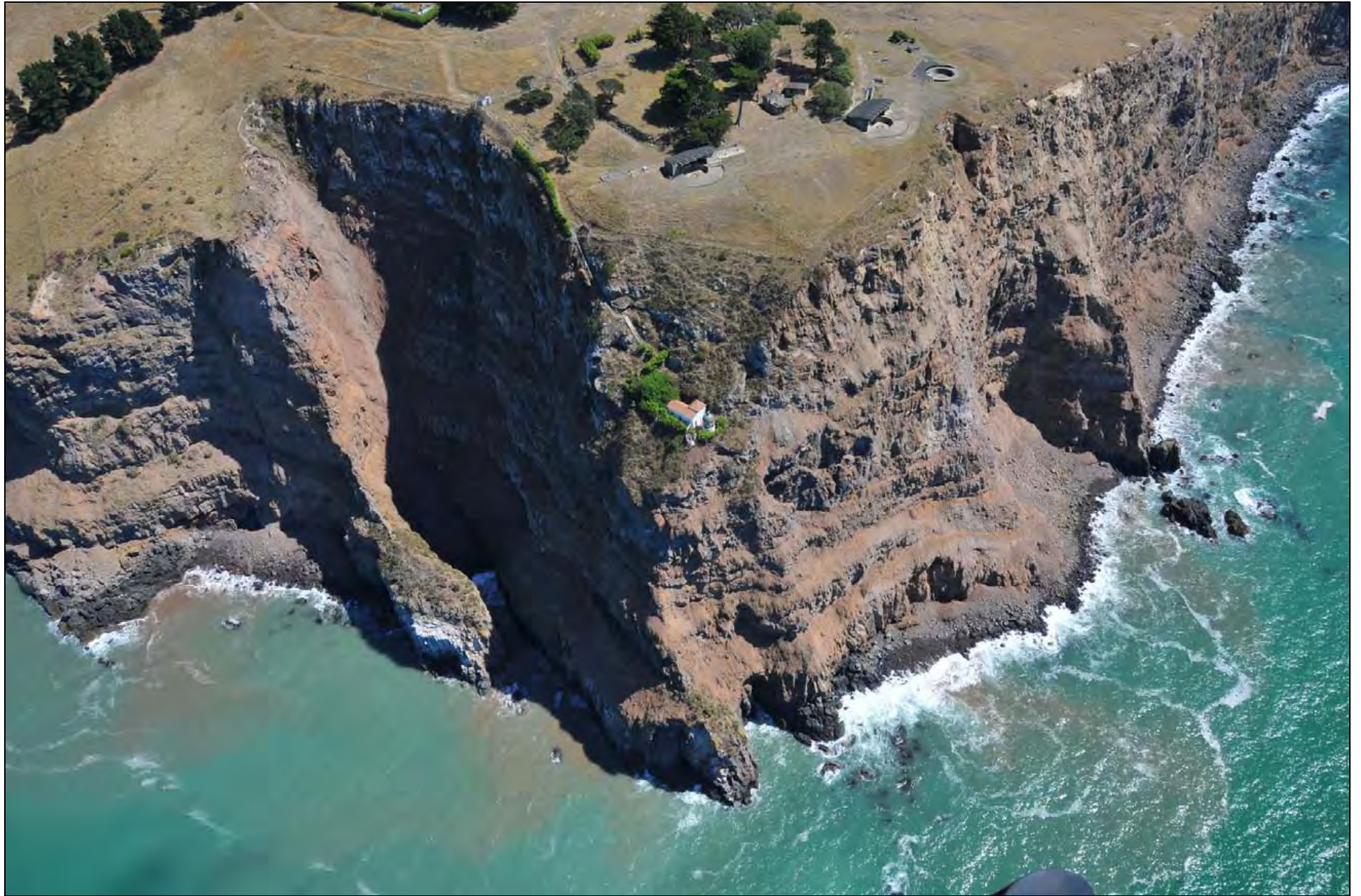
Photo 1. Small rock and debris falls on ~100 m high sea cliff at Godley Head ( GNS Photo-GTH_5622 ).
