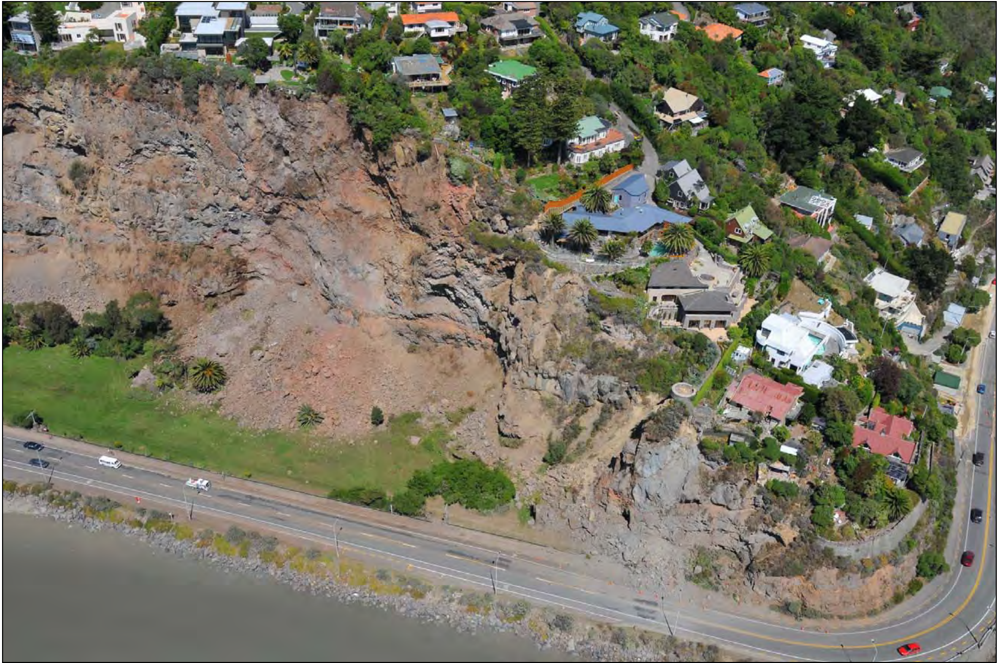
Photo 13. Rock falls below Kinsey Tce on to the Main Rd at the Moncks Bay–Shag Rock headland at Sumner ( GNS Photo-GTH_5753 ).
