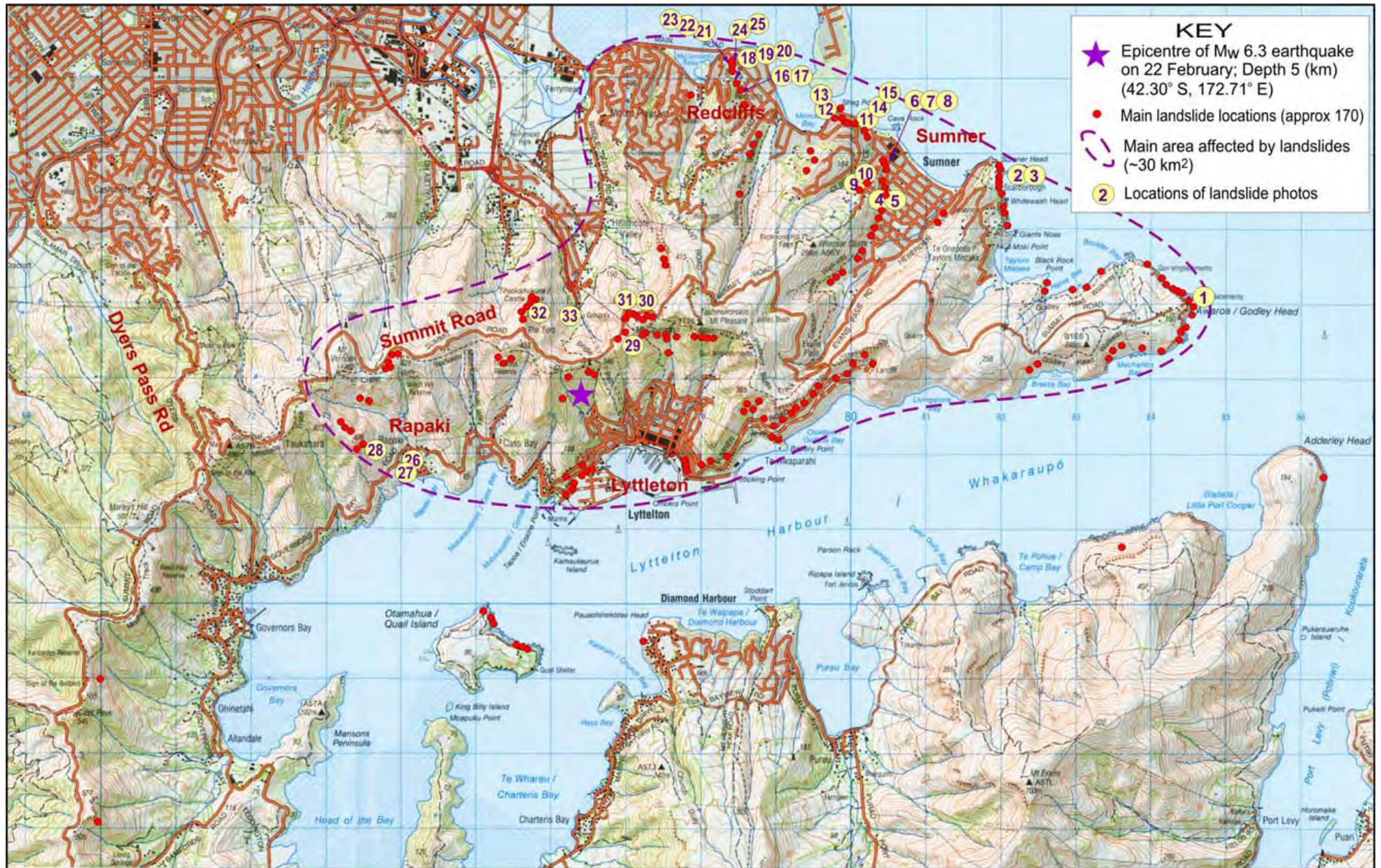
Figure 2. Map showing the distribution of landslides triggered by the 22 February earthquake, the main area affected, and locations of landslide photos.
