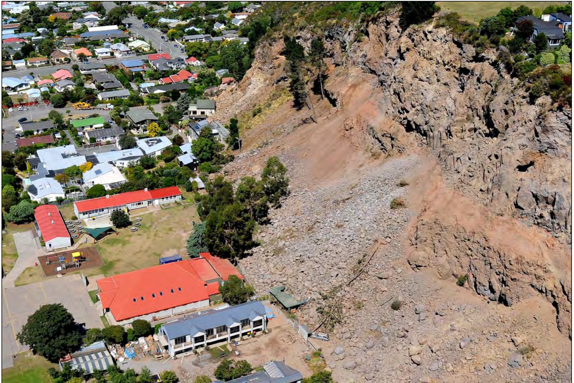
Photo 18. Large rock and debris falls on the ~60 m high cliff face behind Redcliffs School ( GNS Photo-GTH_5801 ).
