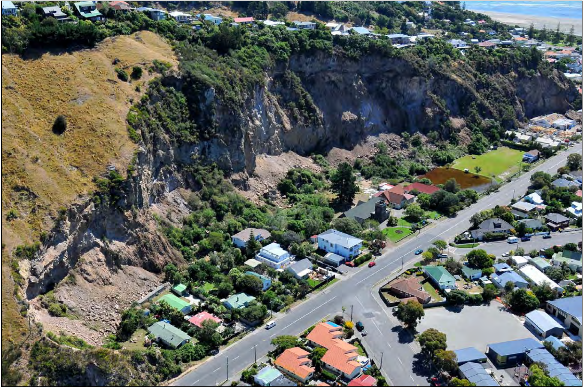
Photo 4. Rock and debris falls on ~50 m high cliff behind houses at the north end of Wakefield Ave, Sumner. This is an old quarry site ( GNS Photo-GTH_5699 ).
