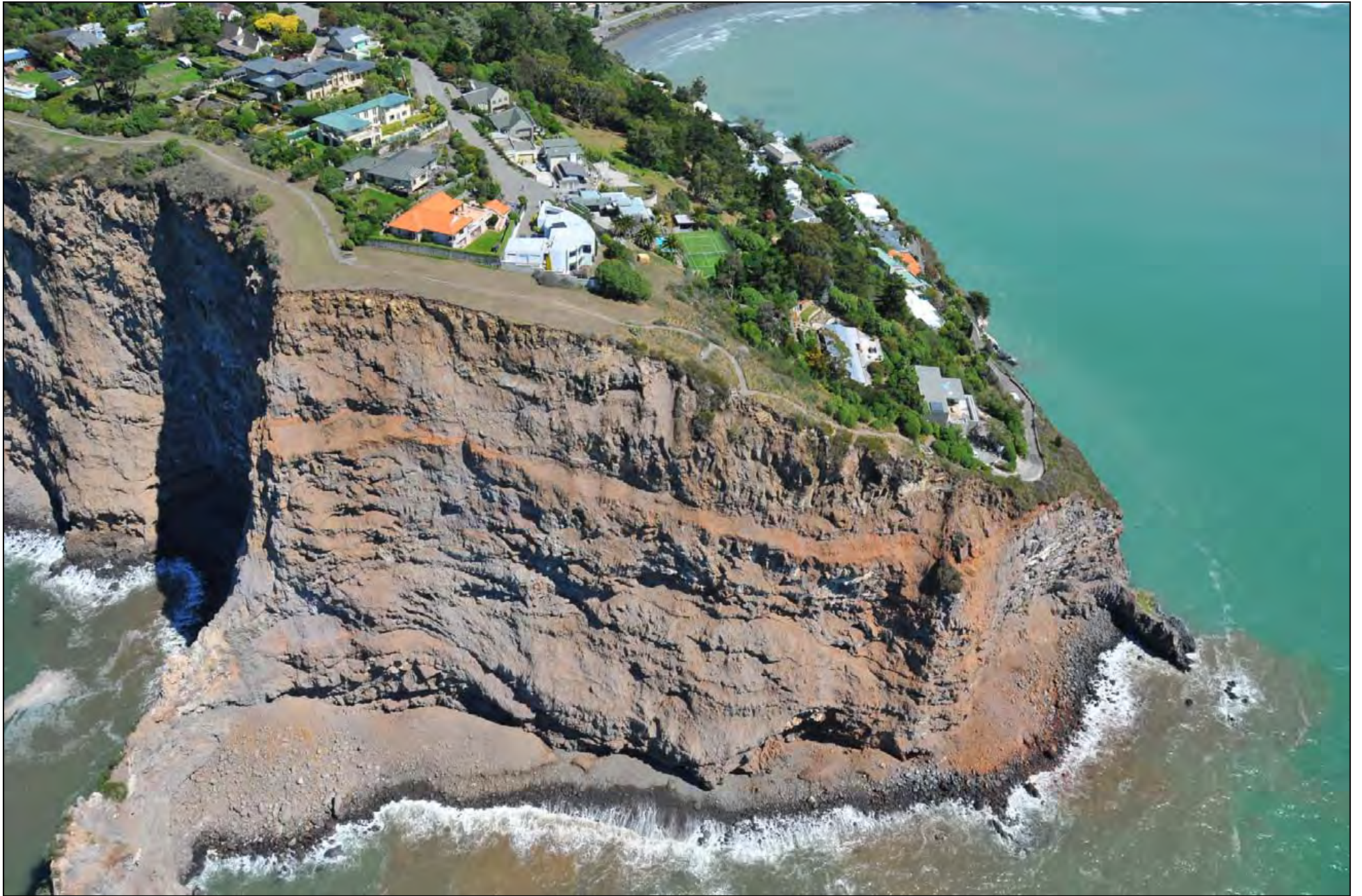
Photo 2. Small rock and debris falls on ~100 m high cliff below Searidge Lane at Sumner Head, Scarborough ( GNS Photo-GTH_5654 ).
