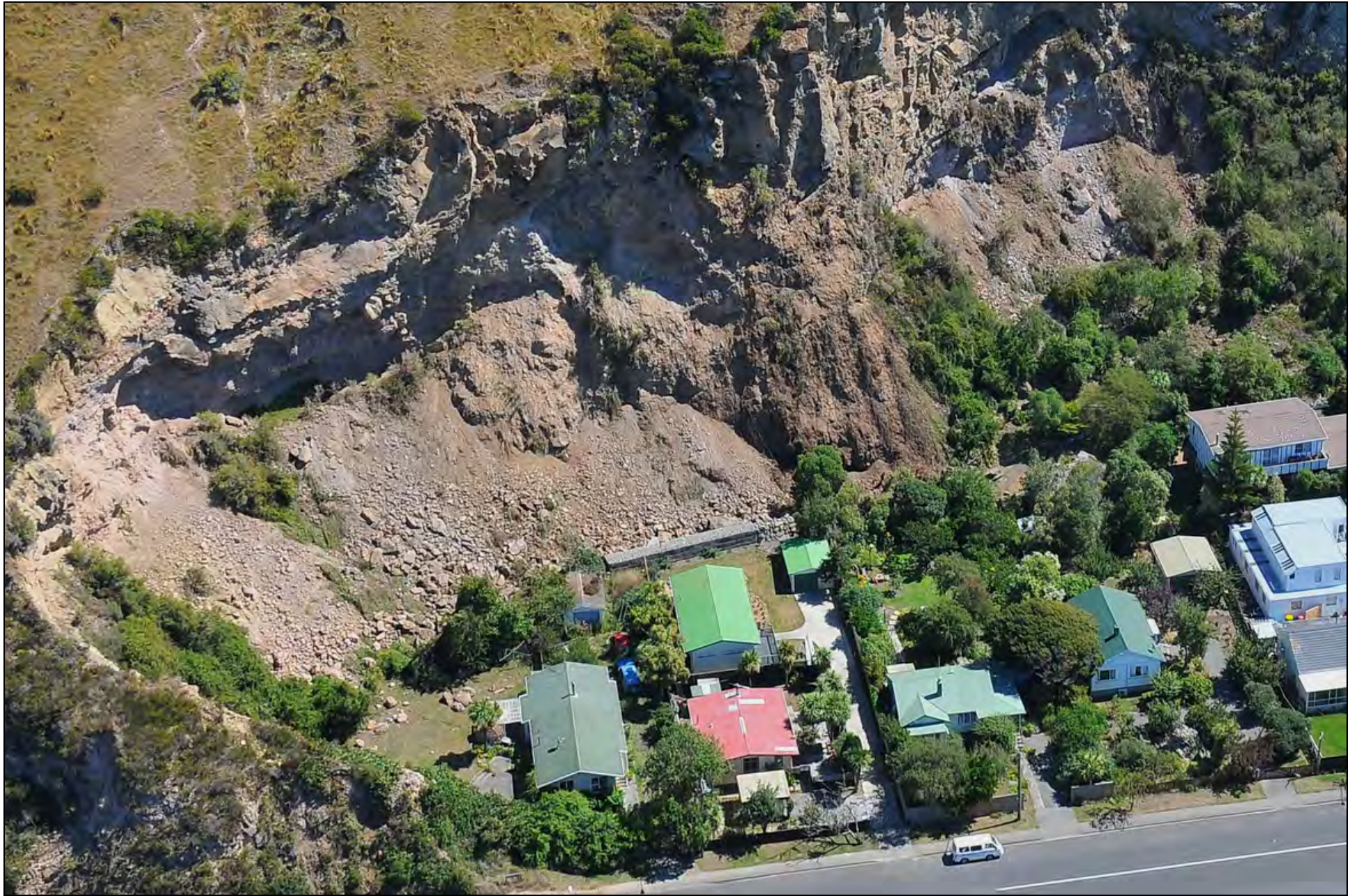
Photo 5. Small rock falls and boulders on gardens close to houses between Arnold and Colenso streets, Wakefield Ave, Sumner ( GNS Photo-GTH_5700 ).
