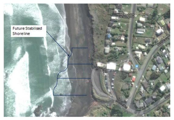
Figure 25 : Diagram of Potential Groins at Port Waikato
