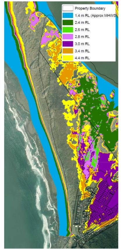
Figure 8: Coastal inundation modelling based on LIDAR Model (Source: Waikato District Council)
