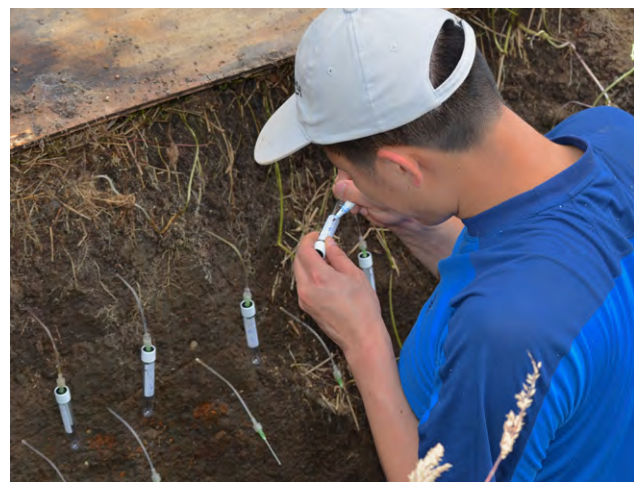
Figure 4.1: Leachate sampling from different soil horizons (Hongtao Zhong) in a soil pit at the PCRP project site
