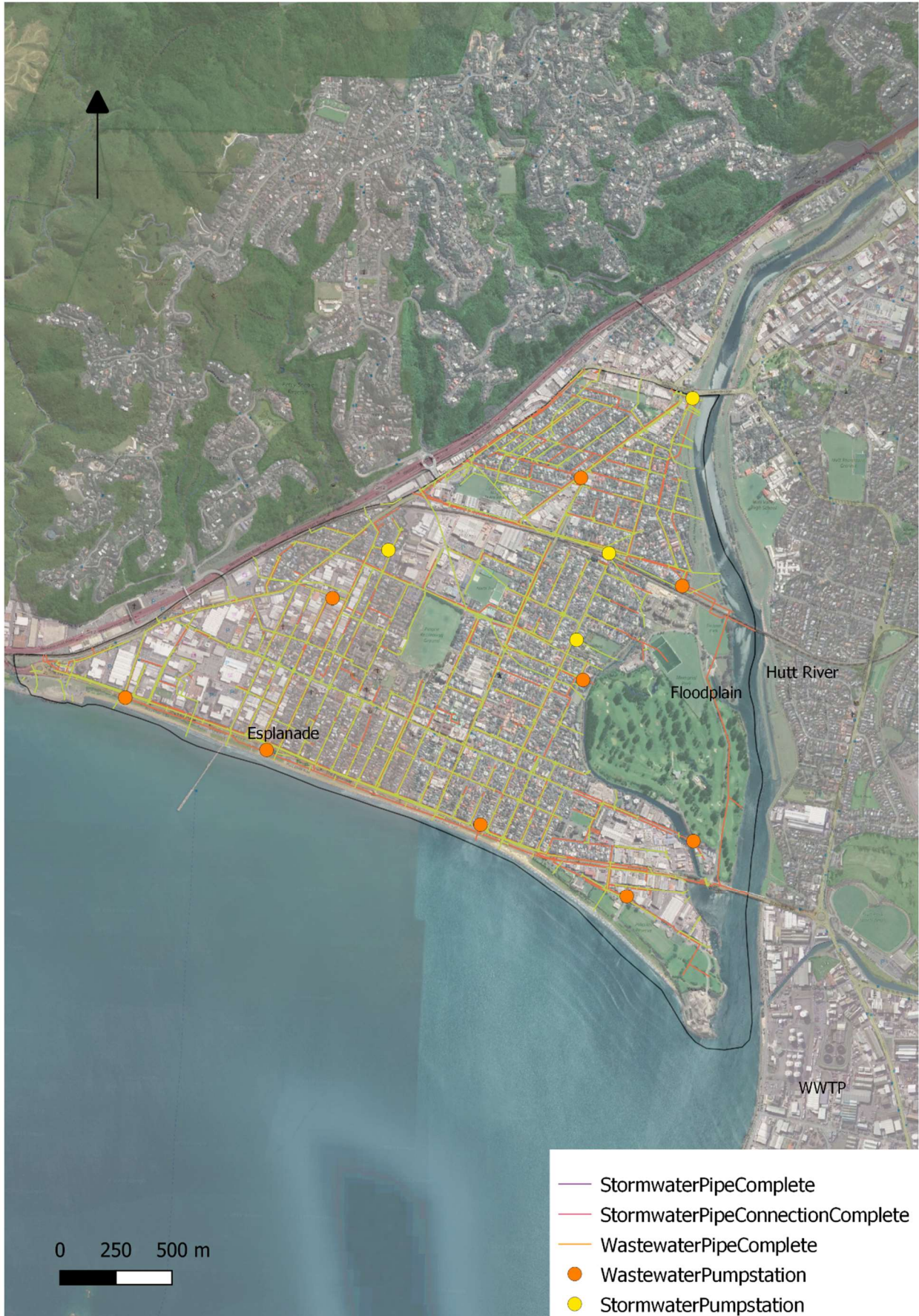
Figure 4: Pumping Stations and Pipe Network Petone
