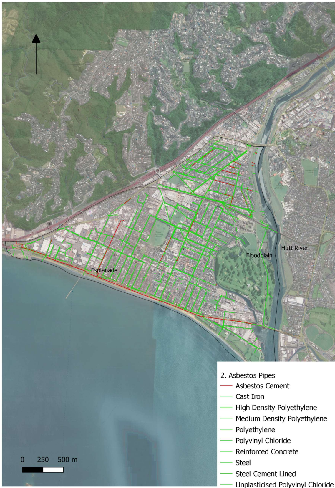
Figure 24: Location of Asbestos Pipes
