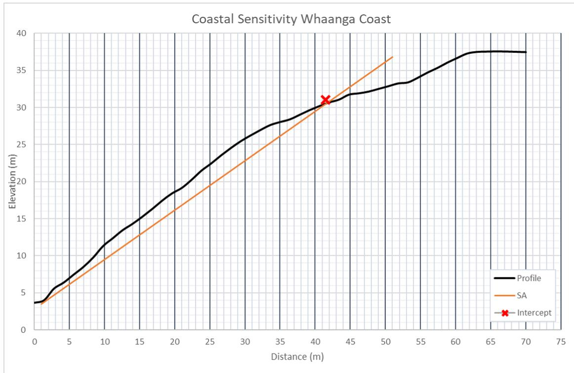
Figure 7: Example of slope based coastal sensitivity area on cliff coastline.
