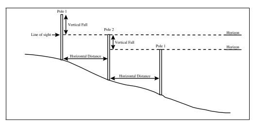
Figure 9 Measurement downslope using Emery Pole technique
