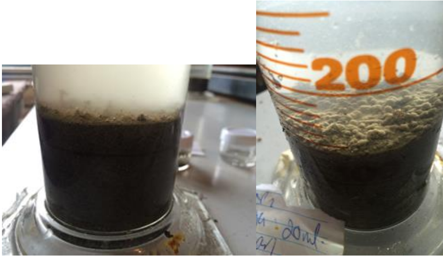
Figure 5.40 (left): Visible aggregations formed after 3 minutes. Figure 5.41 (right): Aggregations were larger, more spherical and covered in a yellow veneer of flocculated particles after nearly 18 hours.
