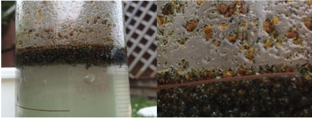
Figure 5.31 (left): Oil slick at the water surface after 2 minutes and 40 secs. Figure 5.32 (right): Close up of the individual tar patches that form the slick.
