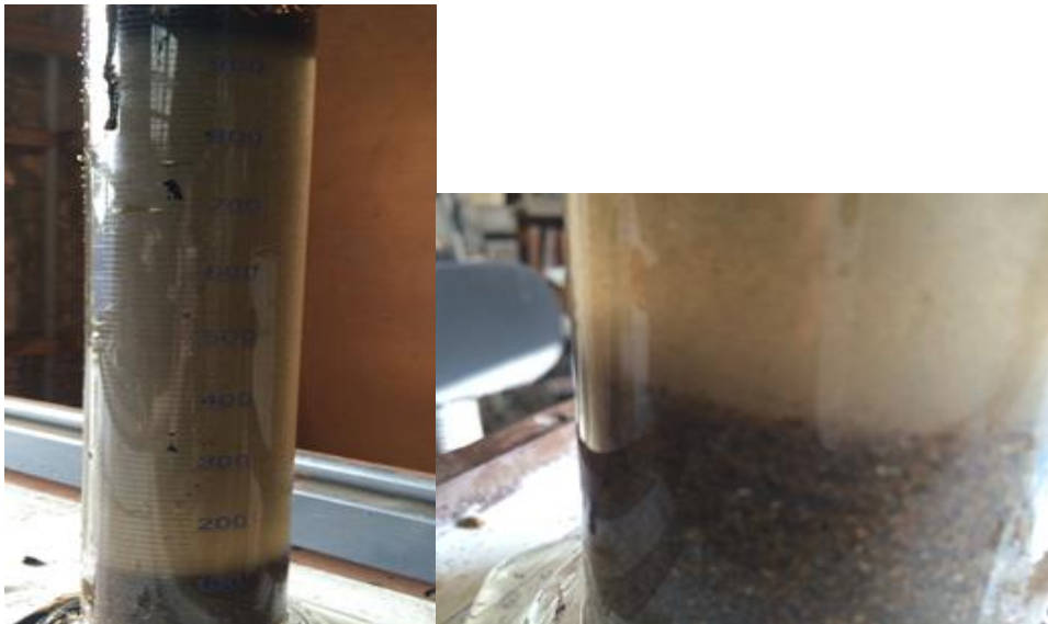
Figures 5.10 (left) and 5.11 (right): After 1 minute, there is a distinctive lighter layer near the base of the water column.
