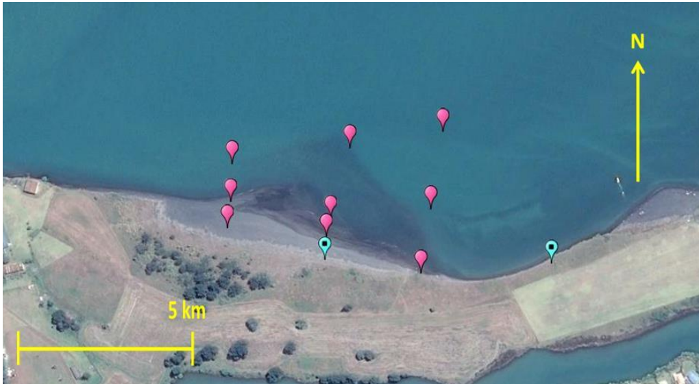
Figure 3.3: Rod locations and control points (CP18 and CP19 in blue) at Wainamu Beach.
