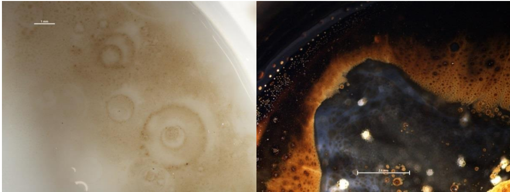
Figure 5.86 (left): Concentric rings coating the container lid. Figure 5.87 (right): Surface slick exhibiting early stages of emulsification.
