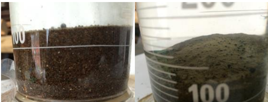
Figures 5.8 (left) and 5.9 (right): Tar balls on the sediment surface after approximately 60 hours and 36 hours respectively.
