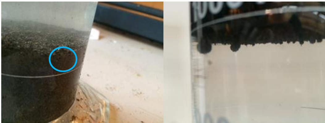
Figure 5.17 (left): Air bubbles and oil droplets on the sediment surface. Figure 5.18 (right): Tar balls distended from the base of the surface slick.
