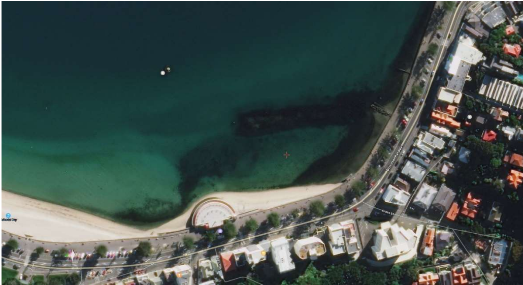
Figure 6.14. The submerged reef at Oriental Bay is designed to maintain beach sand along the eastern part of the beach through wave rotation (Mead and Black, 2001). ( https://satellites.pro/New_Zealand_map#-41.290467,174.795637,19 ).
