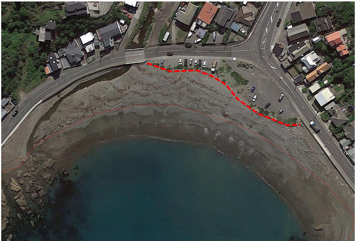
Figure 6.11. Potential rock revetment for Ōwhiro Bay to reduce wave run-up onto the road and threatening properties during extreme events.
