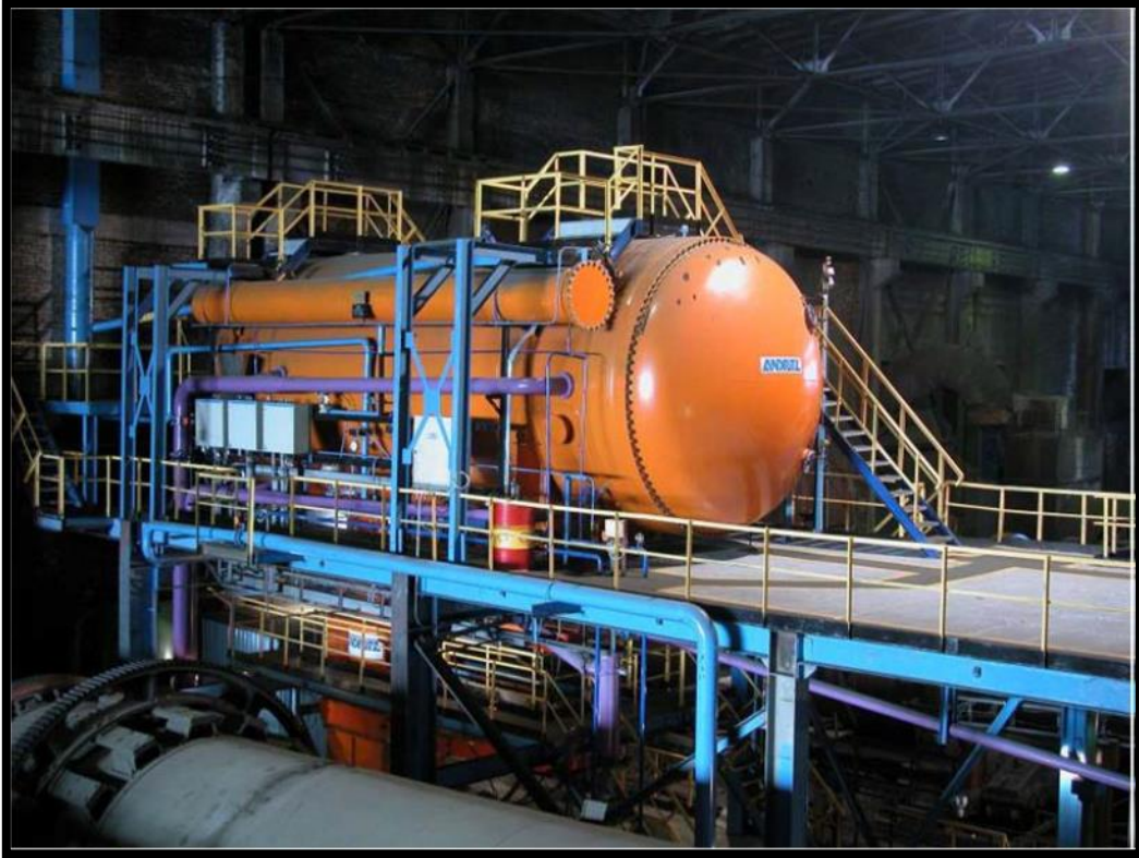
Figure 2.9: Example of the Hyperbaric Pressure Filter
