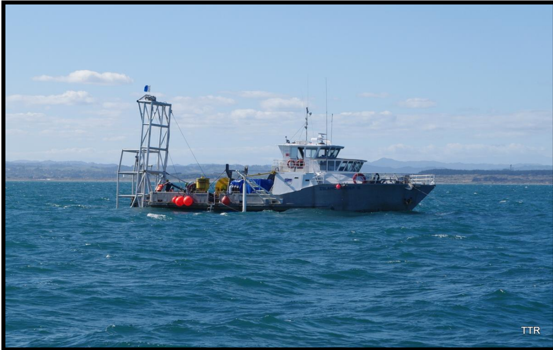
Figure 2.5: The Island Leader II. Used by TTR for offshore drilling in the South Taranaki Bight. Note the structure at the aft of the vessel is the launch and recovery system from which the grade control drill rig will be launched and recovered from.
