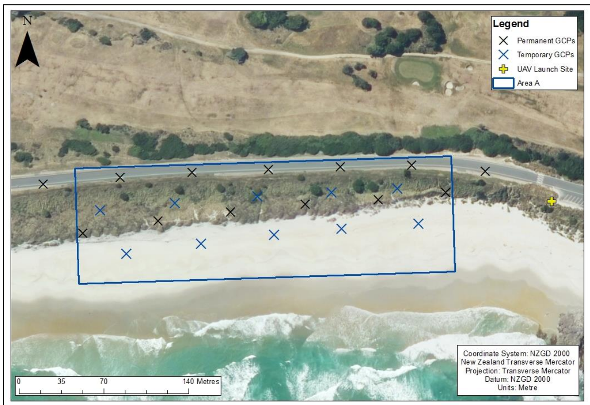
Figure 3.5: The location of the ground control point configuration for the RPAS flight. The permanent points are road markings and fence posts on the dune crest, the temporary points are foam targets placed on the beach.
