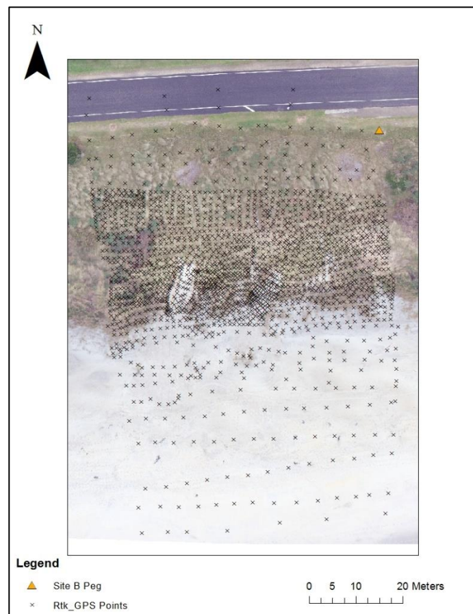
Figure 3.3: The location of each point taken in the RTK-GPS survey. The location of the base station is denoted as ‘Site B Peg’.
