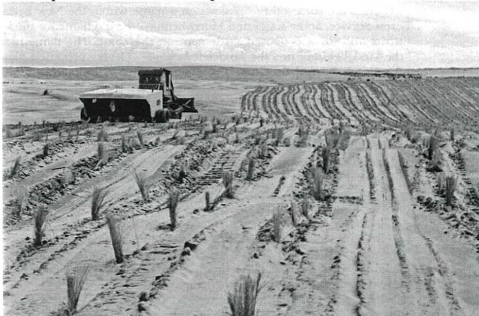
Photo 6 – A 6-Man marram planting machine capable of planting 20 ha of marram grass per day.
